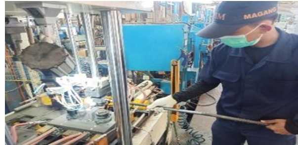
Gambar 13. Proses Trial Casting Piston Gasoline
