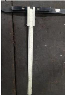
Gambar 7. Depth Caliper
