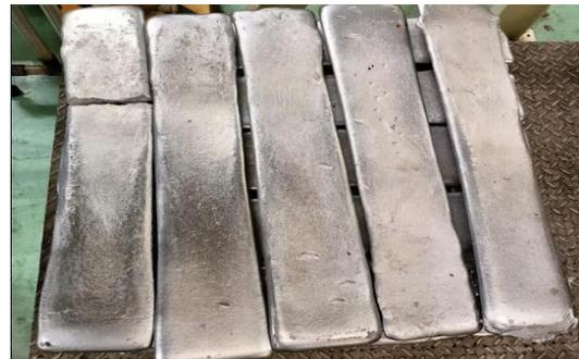
Gambar 11 Material Ingot AC2B
