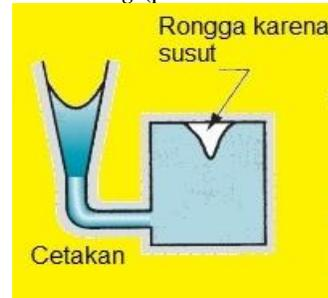
Gambar 3 Ilustrasi Cacat *Shrinkage Porosity*
