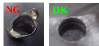
Gambar 4. 4. Jenis Defect Outflow : Hole Function Burry
