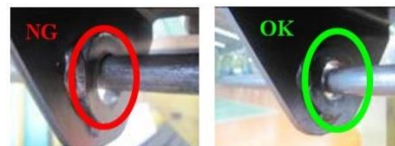
Gambar 4. 6. Jenis Defect Outflow : Pin Sulit Dipasang di Hole Bracket Spring
