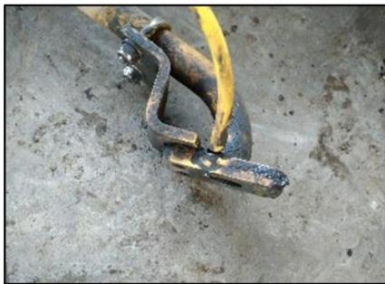
Gambar 1. *Tube Fill Transmission* patah
