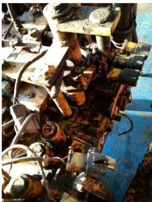
Gambar 2. *Inching Potensiometer* Aus
