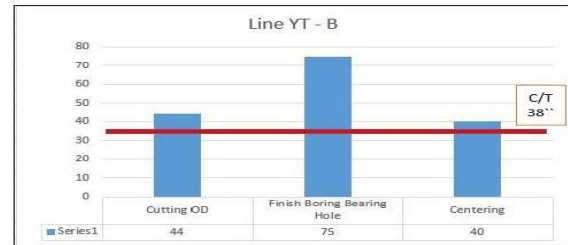
Grafik 4.4 Cycle Time Line Yoke Tube A dan Yoke Tube B after improvment
