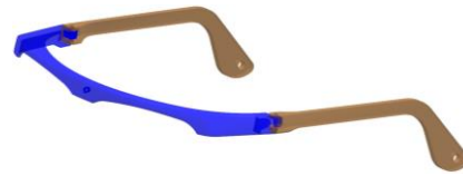
Gambar III. 1 Model 3D produk safety glasses frame (sumber: UPT Design dan metrologi, 2015)
